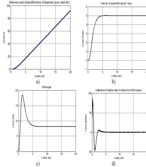
Figure 2. Results of simulation of motion control along the  $Y$ -axis: a) following command signal (black line) by quadrotor (grey, dash-dot line), b) transient process of velocity, c) transient process of roll angle, d) transient process of rotation rate increment of electromotor.
