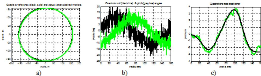
Figure 5. Simulation of the quadrotor path following in the disturbed atmosphere: a) quadrotor path (grey, dashed line) and reference track (black, solid line) in m, b) roll angle (black line) and pitch angle (grey line) in , c) cross-track error in the calm atmosphere (in m, black line) and the same error in the disturbed atmosphere (in m, grey line).
