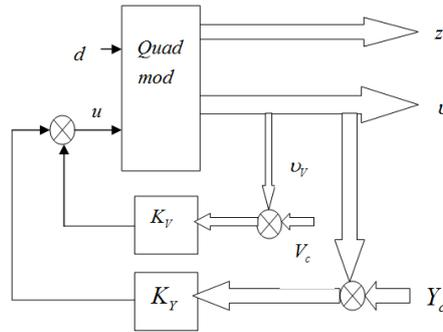
Figure 1. Scheme of the Y-axis control system.
