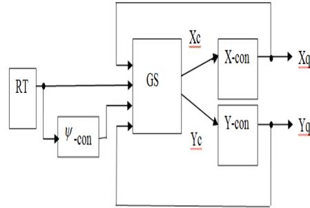
Figure 3. Block diagram of path following system in the horizontal plane.
