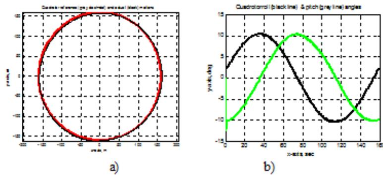
Figure 4. Simulation of the quadrotor path following in the calm atmosphere: a) quadrotor path (grey, dash-dot line) and reference track (black, solid line), b) roll angle (black line) and pitch angle (grey line) in *deg*.
